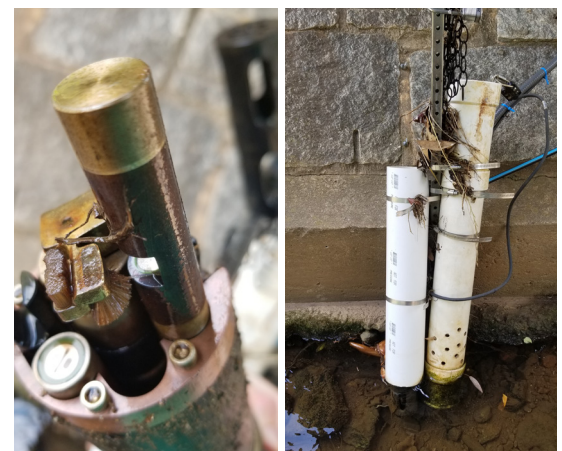
EXO Sonde with water temperature, conductance, pH, DO, turbidity, chlorophyll, and phycocyanin sensors.
